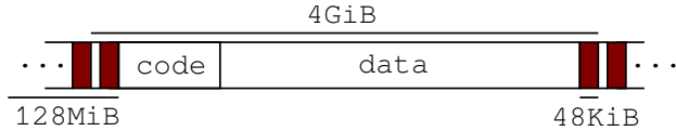
Figure 1. The layout of an LFI sandbox (not to scale). The base address must be aligned to a 4GiB boundary. Guard regions of size 48KiB are shown in red. The code must be at least 128MiB away from any executable region in neighboring sandboxes. One page is reserved between guard regions for the runtime call table, discussed in Section 4.4.
