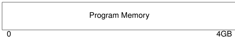
Figure 9.1: Flat Memory Model
