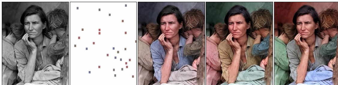
Figure 3.1: Our proposed method colorizes a grayscale image (left), guided by sparse user inputs (second), in real-time, providing the capability for quickly generating multiple plausible colorizations (middle to right). Photograph of Migrant Mother by Dorothea Lange, 1936 (Public Domain).
