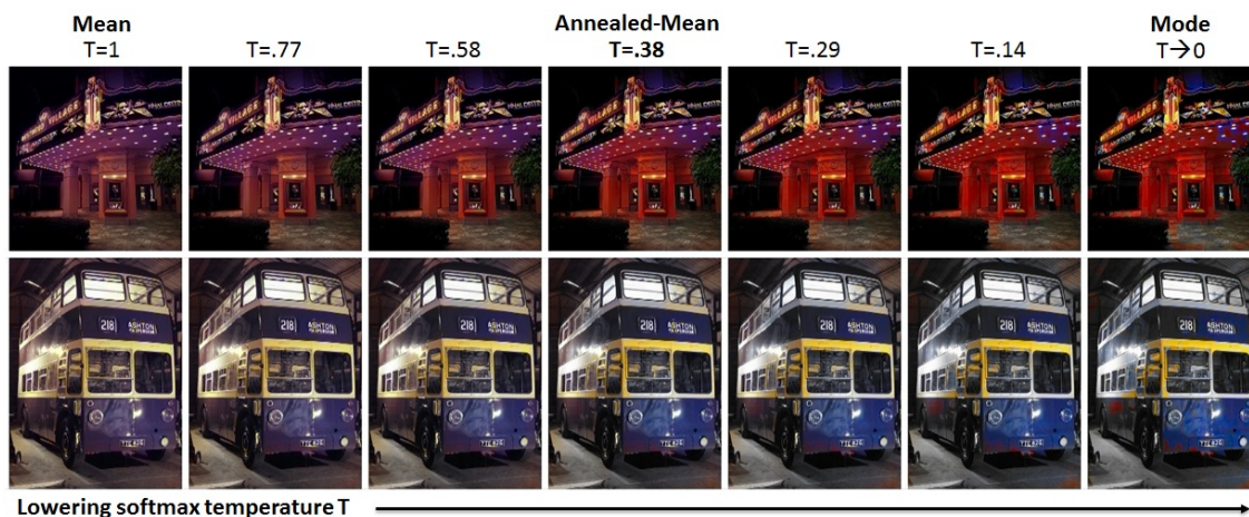
Figure 2.4: The effect of temperature parameter T on the annealed-mean output (Equation 2.5). The left-most images show the means of the predicted color distributions and the right-most show the modes. We use T = 0.38 in our system.
