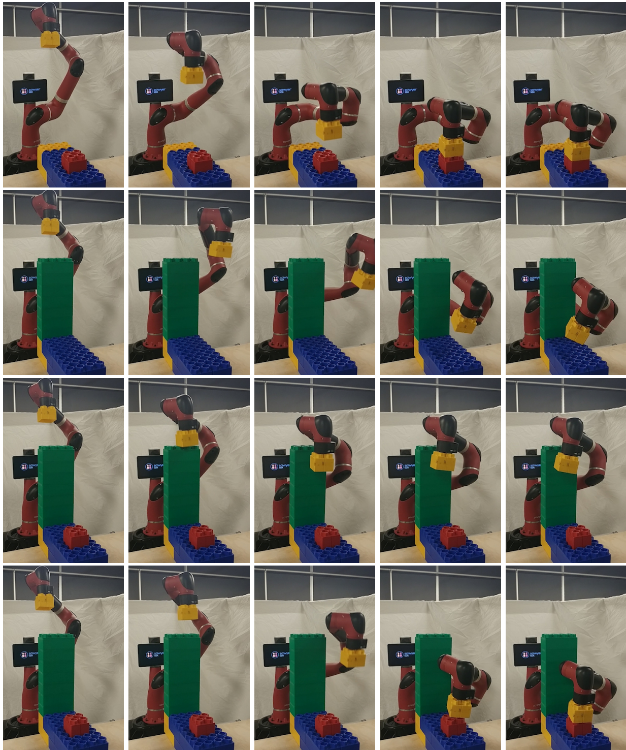
Figure 6.3: To illustrate compositionality on physical hardware, we trained the Sawyer manipulator to stack Lego blocks together (first row) and to avoid an obstacle (second row). The stacking policy fails if it is executed in the presence of the obstacle (third row). However, by combining the two policies, we get a new combined skills that solves both tasks simultaneously and is able to stack the blocks while avoiding the obstacle.
