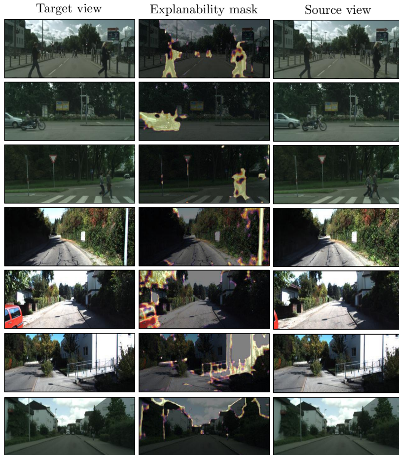
Figure 5.11: Sample visualizations of the explainability masks. Highlighted pixels are predicted to be unexplainable by the network due to motion (rows 1–3), occlusion/visibility (rows 4–5), or other factors (rows 7–8).
