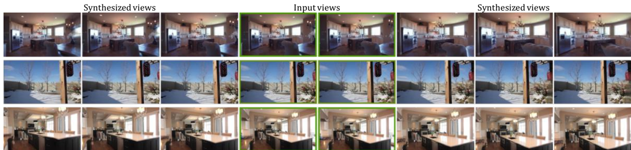
Figure 6.6: Sample view extrapolation results using multiplane images . The central two frames (green) are the input to our network, and the inferred MPI is used to render both past and future frames in the same video sequence.
