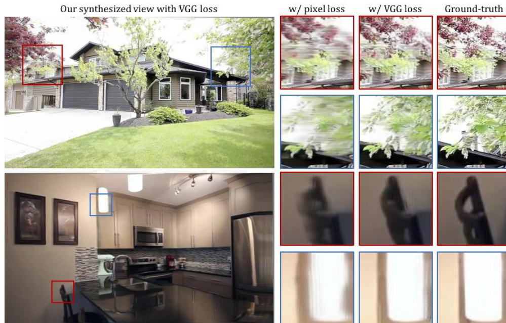
Figure 6.8: Comparison between the models trained using pixel reconstruction loss and VGG perceptual loss. The latter better preserves object structure, and tends to produce sharper synthesized views.
