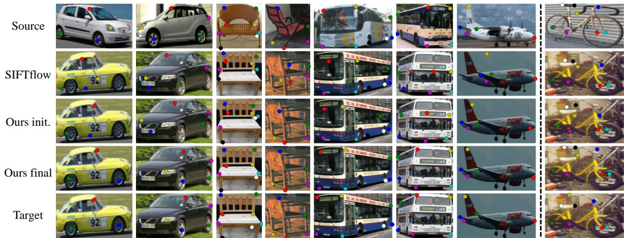
Figure 3.4: Comparison of keypoint transfer performance for different methods on example test image pairs. Overall, our consistency-supervised network (second-to-last row) is able to produce more accurate keypoint transfer results than the baselines. The last column shows a case when SIFT flow performs better than ours.
