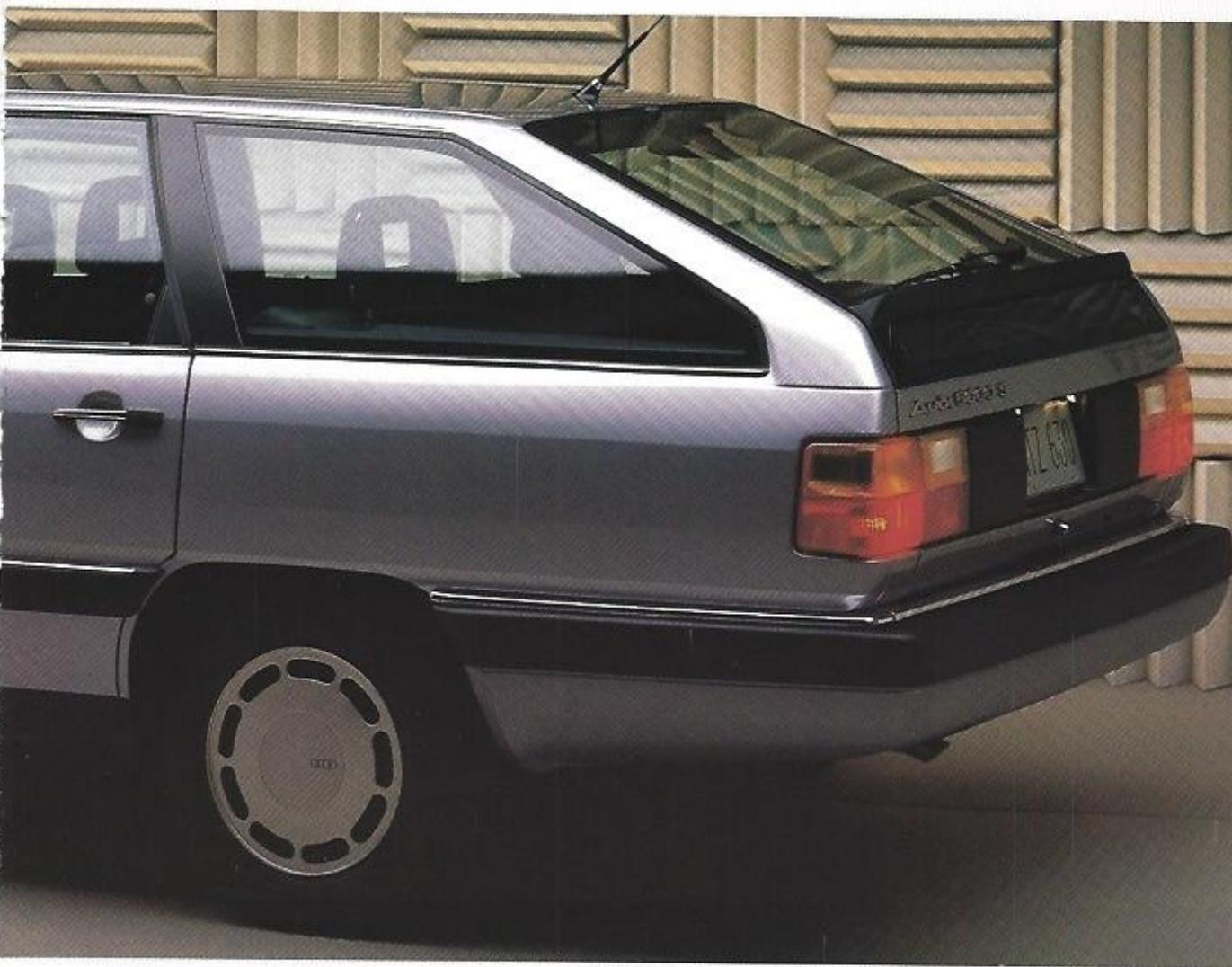
Because the most important cargo that it will carry is your loved ones—and especially children—Audi engineering builds safety into the 5000S Wagon. A rigid sheet steel frame construction surrounds the passenger cell. Wide, steel-reinforced molding runs
