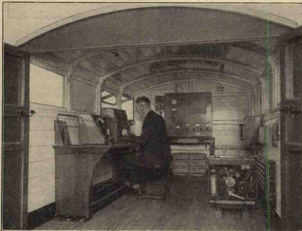
RADIO AT CIVIL AERODROMES. An increasing number of civil air ports are now equipped with radio ground stations. The photograph shows one of the motor "trailers," fitted with Marconi transmitting and receiving apparatus, as installed at the Hull, Belfast and Portsmouth air ports.
