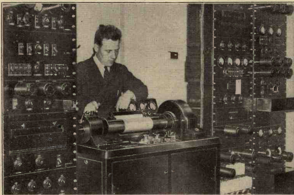
The Marconi Facsimile transmitter at the Central Telegraph station in London of Cable and Wireless Ltd. A regular phototelegraphy service has been opened between Australia (Melbourne) and London. A picture 9 in. by 9 in. occupies half an hour in transmission. The photoelectric cell is operated by light reflected from the surface of the photograph.
