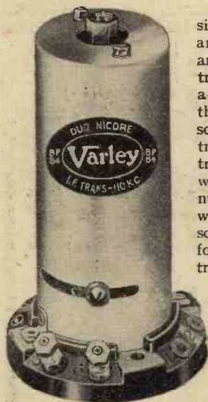
Varley Duo Nicore 110 kc/s IF transformer, showing band-width control screw and trimmer adjusters on top.
