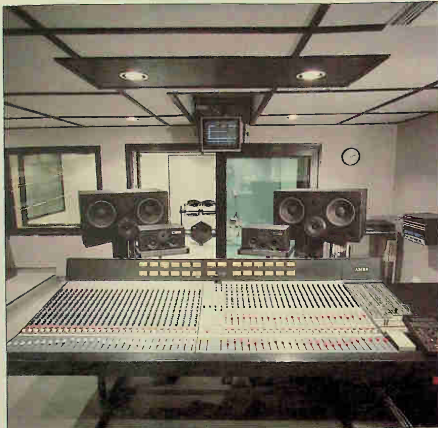
THE CONTROL room: DDA AMR 24 mixing consale with 52 channels Optimix disc automation.
