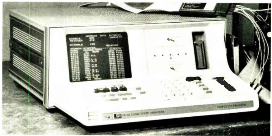
Lots to say. Readout of mnemonic operating codes that match up with the actual program steps makes debugging much easier with HP's $5,000 microprocessor analyzer (p.32).
