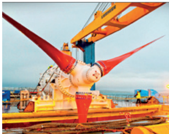
The blades and nacelle of the HS1000 tidal turbine in transportation to the European Marine Energy Centre in Orkney
