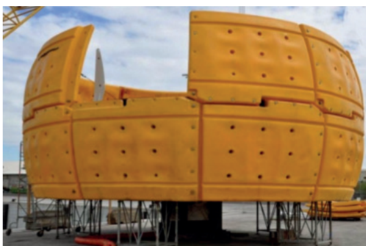
Assembly of the Buoyant Actuator at La Reunion. CETO 4 (Average output estimated at 180kW over 20 minutes)
