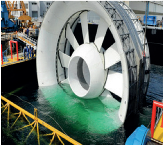
16m turbine being placed onto a deployment vessel at Brest, France
