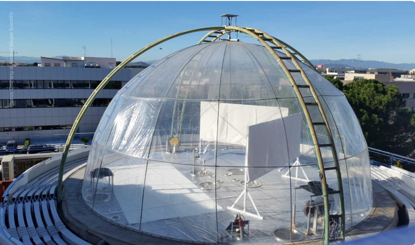
Testing of new Aerosol Magee Scientific instruments at EUPHORE in Valencia, Spain, a major international outdoor simulation chamber for research on atmospheric pollution, air pollutant effect, forest research, meteorology and climatology.
