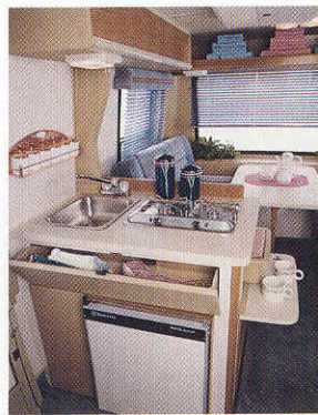
For meals and snacks, the efficient galley has a stainless steel sink, two-burner range top, two-cubic foot refrigerator and lots of storage space.
