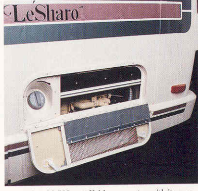
The optional 2,500 watt Kohler generator, with its own 8-gallon fuel tank, offers convenient power when a plug-in is not available.
