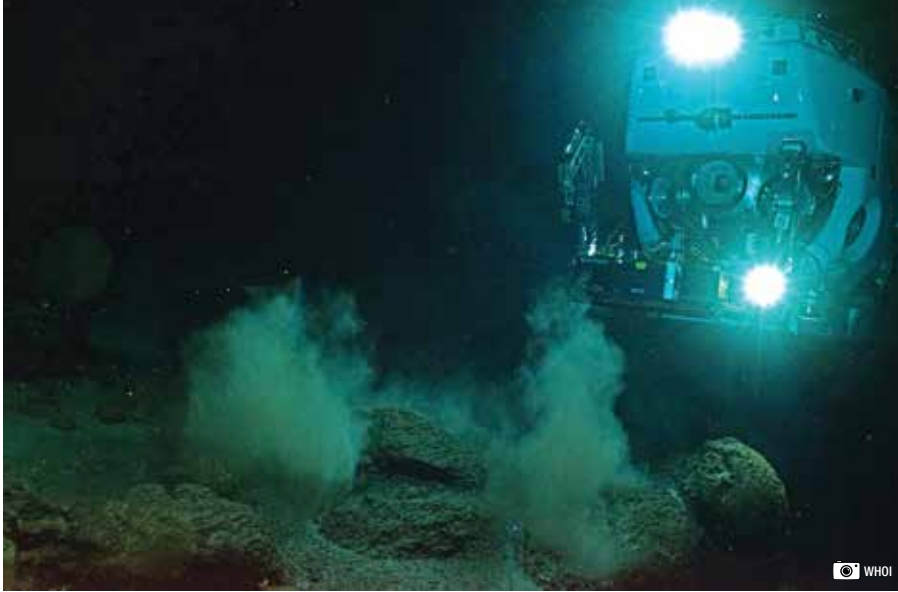
Figure 3: Alvin's new position control system represents a significant improvement to the vehicle's ability to support scientific operations. Alvin is now capable of performing very accurate sonar mapping and photo-mosaic missions, precision transects over long distances and stable position holding near bottom sampling sites.
