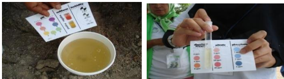
Pemantauan Parameter (pH, coliform, turbidity, dissolved oxygen, phosphate, nitrate) Kualiti Air Guna Test Kit
