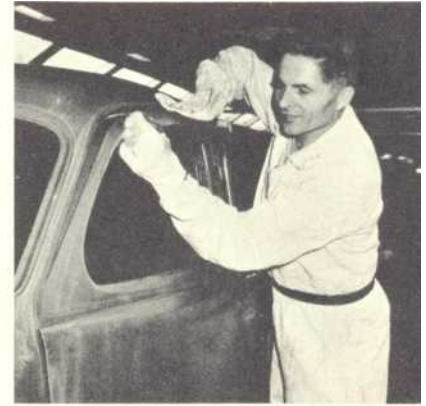
Inspection of enamel base coat after sanding.
