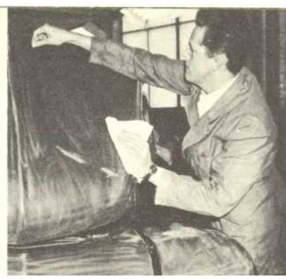
The painting department: inspection of priming after watersanding.
