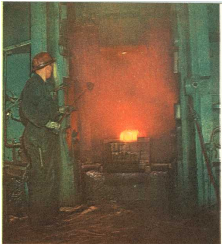
Finishing crankshaft forgings for Volvo in a duplex hammer which develops 290,000 foot-pounds.
