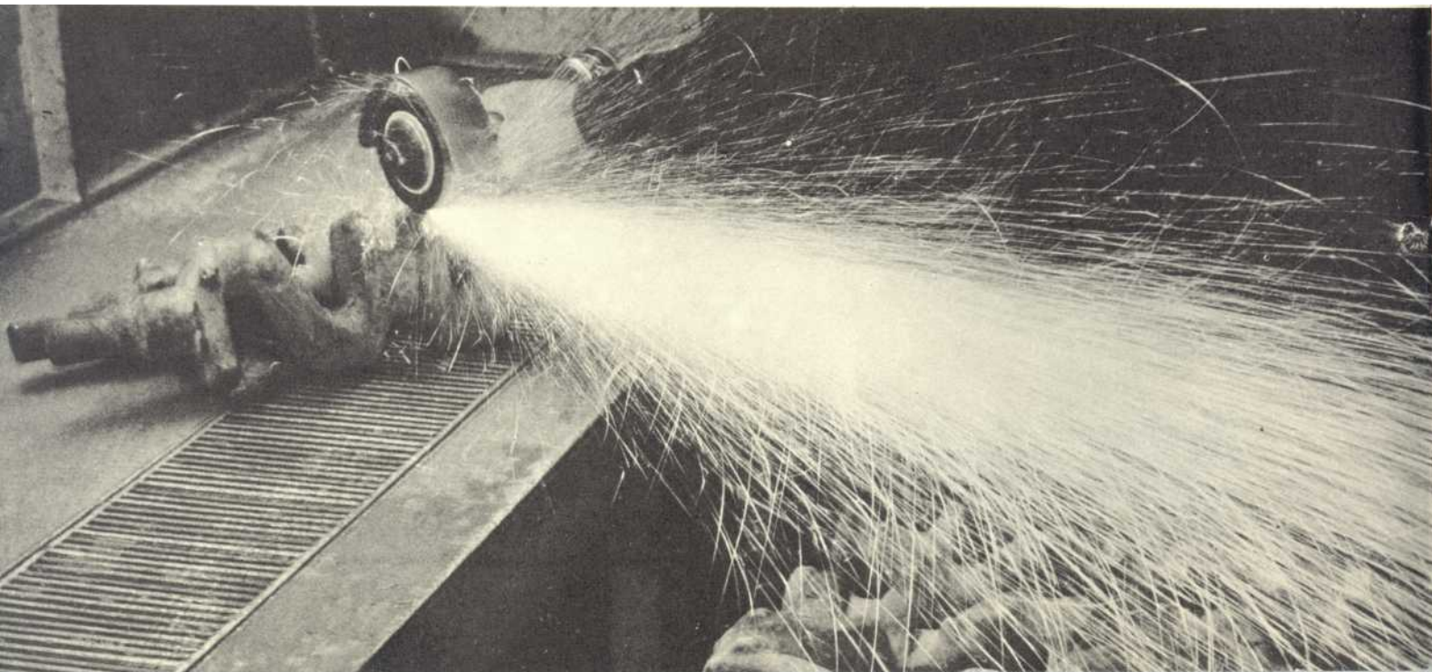
Bofors makes forgings for Volvo crankshafts, gears, and other parts. These blanks are inspected meticulously for correct form and structure, and given a rough machining before shipment.
