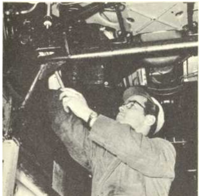
Inspection of rear axle housing and other sub-chassis elements for secure driving.
