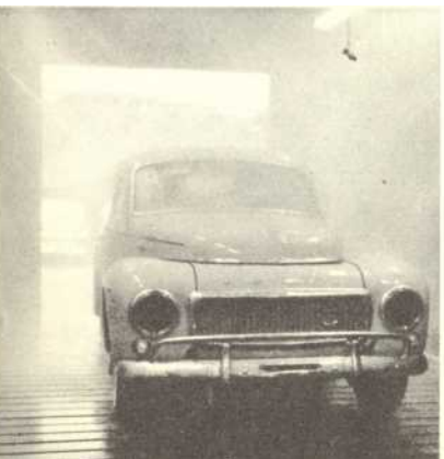
The water test. If the car gets through this high-pressure water dunking, it's not likely to leak later.
