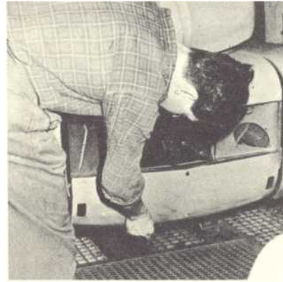
Inspection of enamel base coat after spraying.
