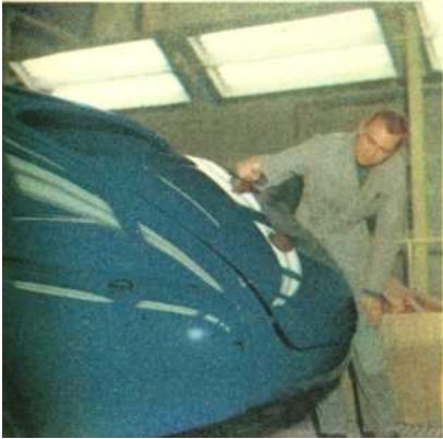
Inspection of enamel top coat.
