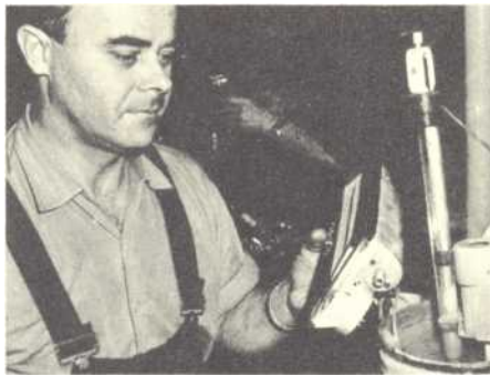
Inspection of coolant thermometer for correct reading.
