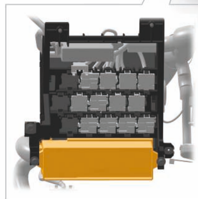
Fuse holder on the front side of the plastic housing – bottom
