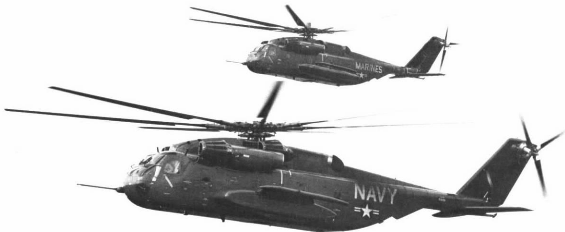
Photo courtesy of Sikorsky Aircraft Division, United Aircraft Corporation Two CH-53Es, one with Navy and the other with Marine markings, fly in formation. The three-engine CH-53E can lift its own weight.
