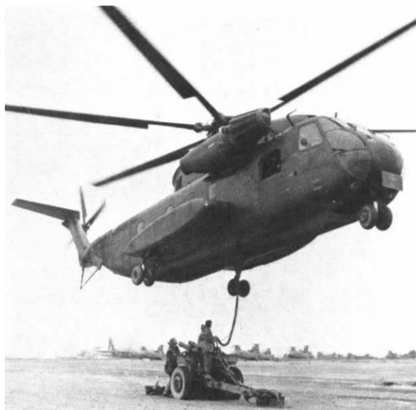
USMC Photo A422527 Before being sent to Vietnam, the CH-53s had large filters installed on the air intake of the engines.
