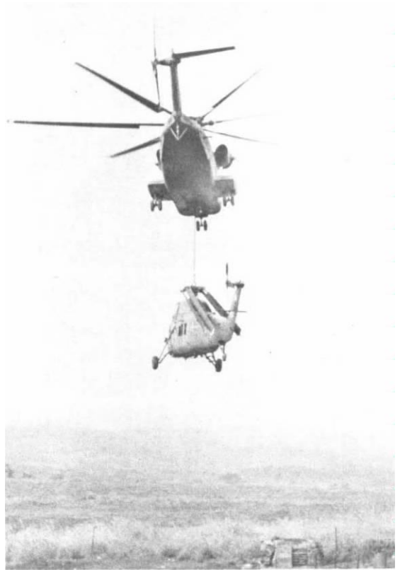
USMC Photo 3d-6-3471-67 A CH-53 lifts a disabled UH-34 out of Con Thien in northern I Corps in 1967. The CH-53A had enough power to lift a "Huss" with the rotor blades on.
