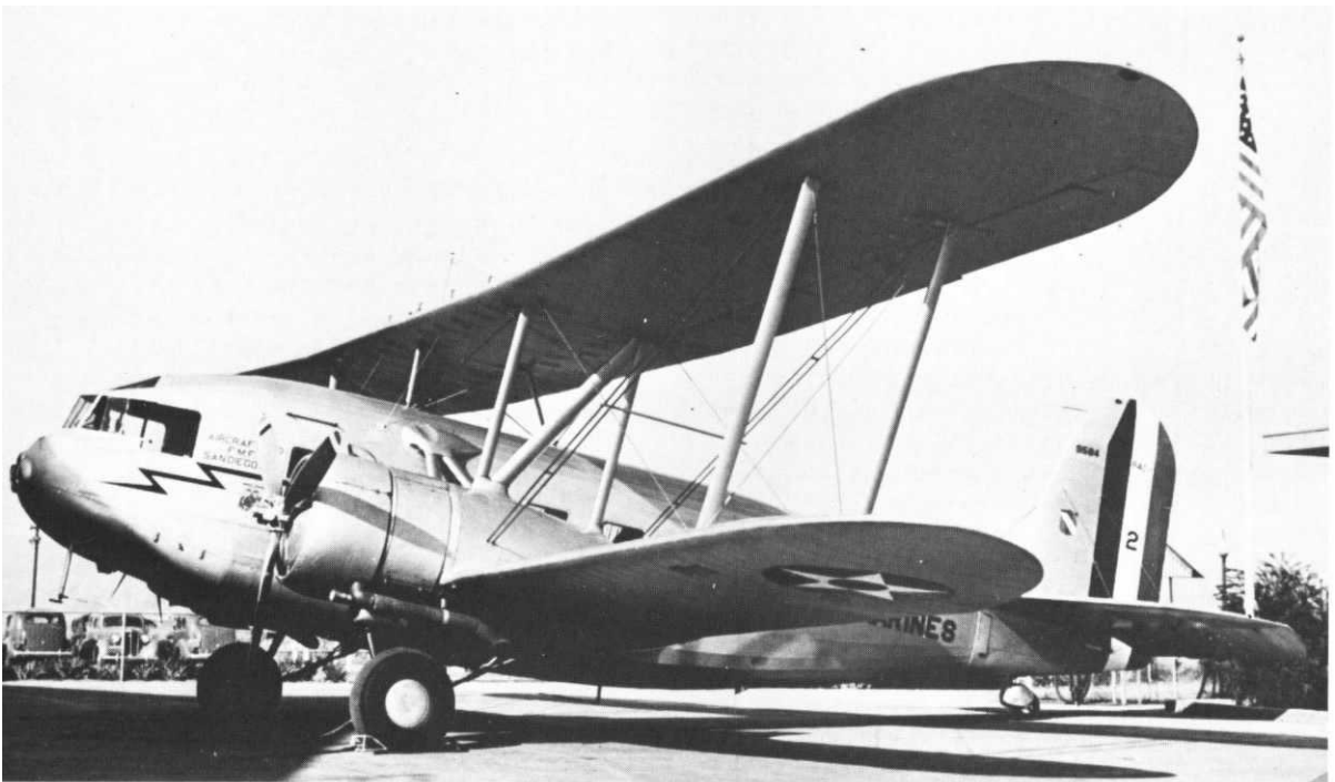
Marines received new transports during the 1930s, including this Curtiss-Wright R4C-1 "Condor" transport in 1937 which had a crew of two and could carry 10 passengers. (Marine Corps Photo 517615).
