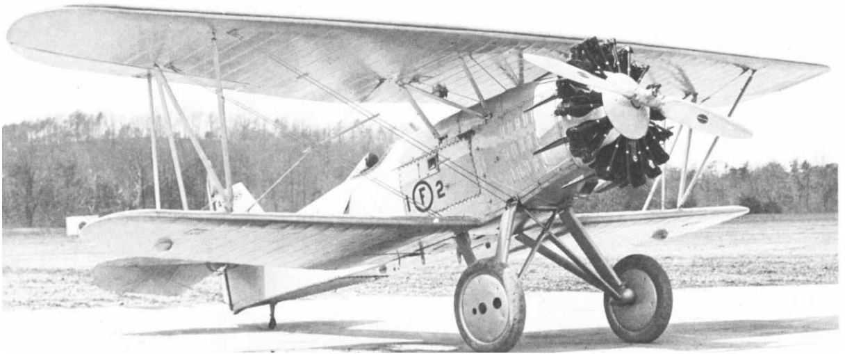
A Curtiss F6C-4 Hawk in 1928. The exposed cylinders of the air-cooled radial engine contrast with the earlier liquid-cooled models. (Marine Corps Photo 515095).
