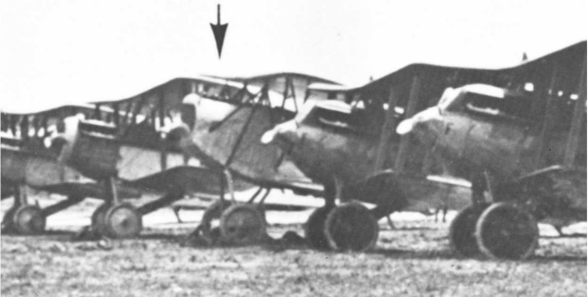
Arrow indicates a Fokker D-7, one of two D-7s to fly with the Marine Corps. The D-7s were captured during World War I. This inspection lineup including VE-7s and MB-3s is at Quantico in 1922. (Photo courtesy Goodyear Kirkham collection).
