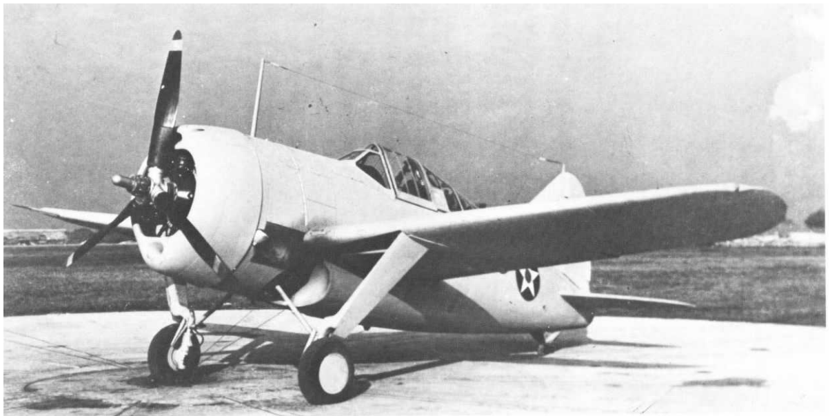
The Marines' first all-metal monoplane fighter, the Brewster F2A-3 "Buffalo." (Marine Corps Photo 304388).
