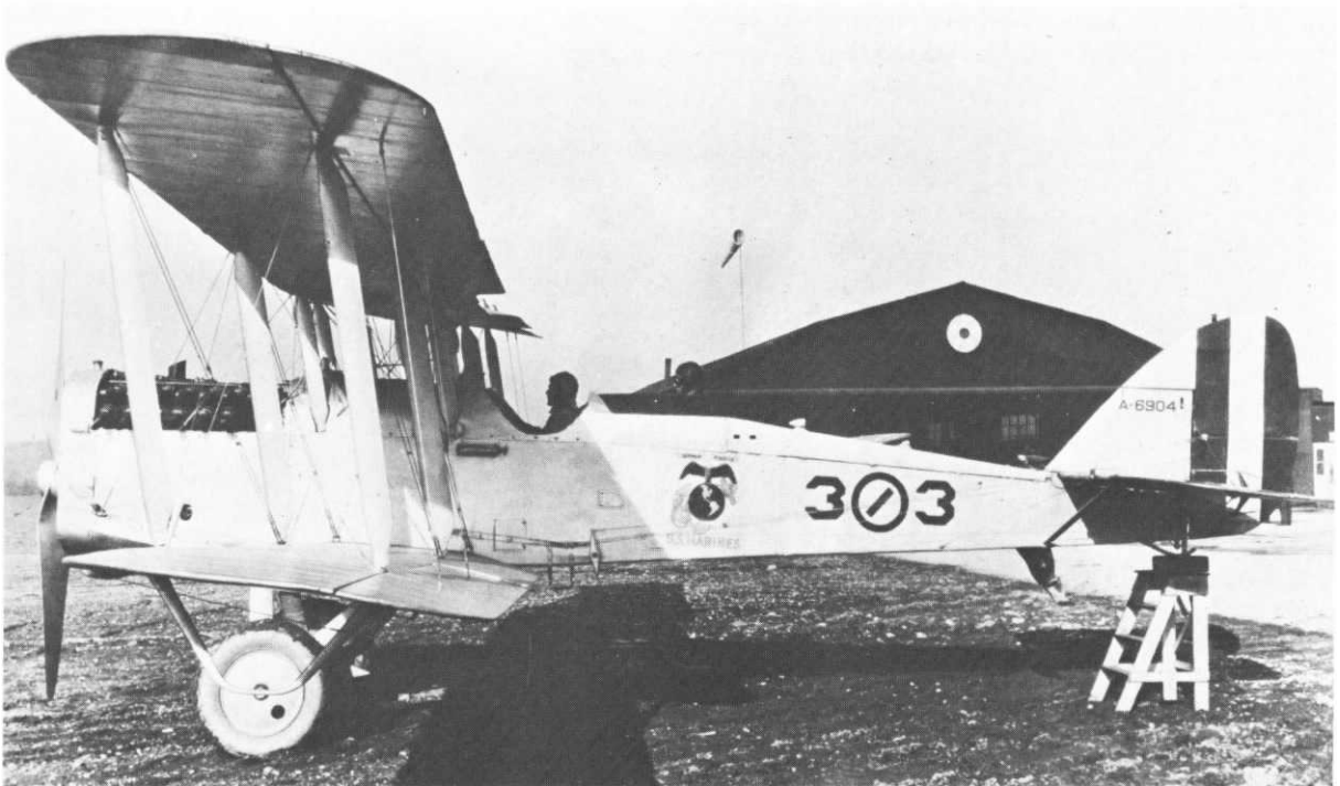
The DH-4B appeared in many guises, including this O2B-1 of VO-3M (Observation Squadron 3) with the 1st Aviation Group in 1921, which served the Marines as an observation and attack plane. (Nat Archives RG 127-G Photo A402979).
