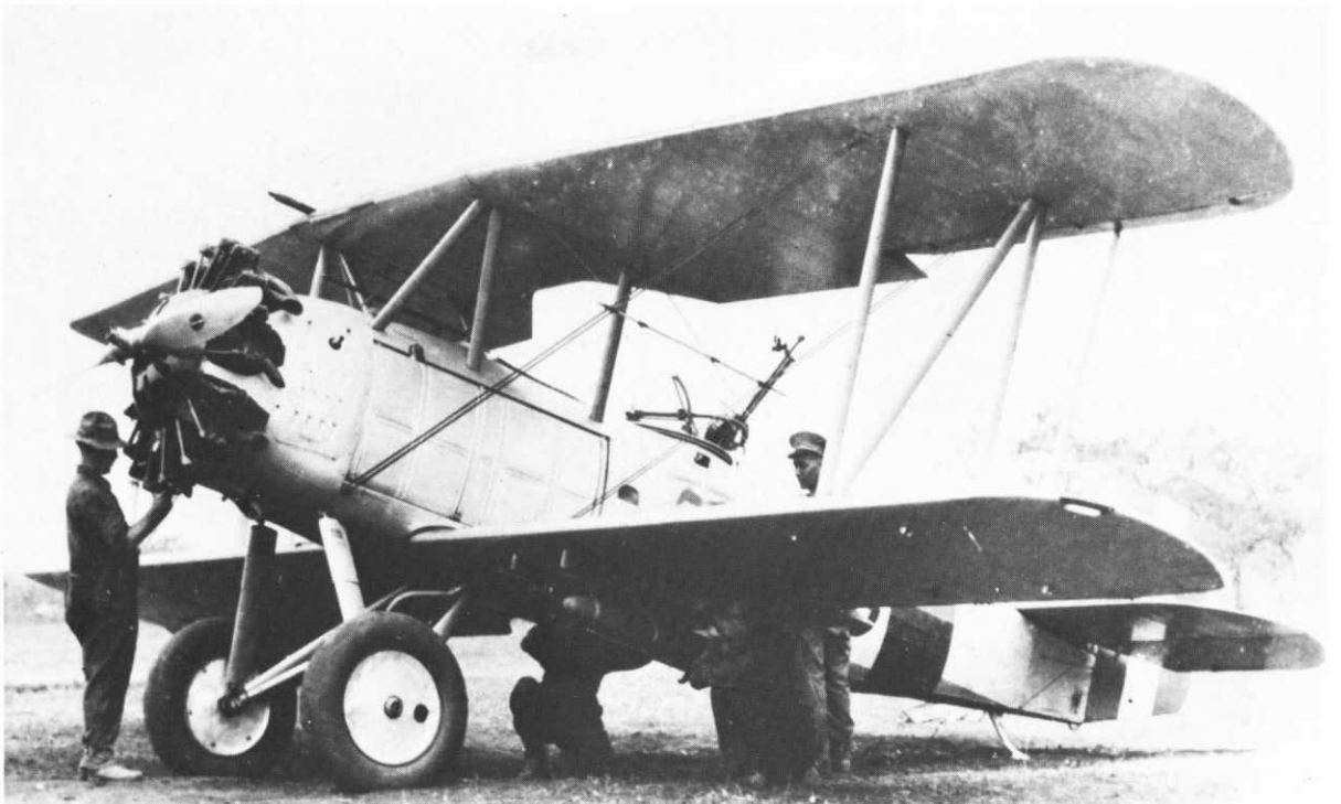
One of two O2U-1 "Corsairs" flown by Lieutenant Schilt at Quilali in 1929. The oversize DH-4B wheels dominate the undercarriage. (Marine Corps Photo 529590).
