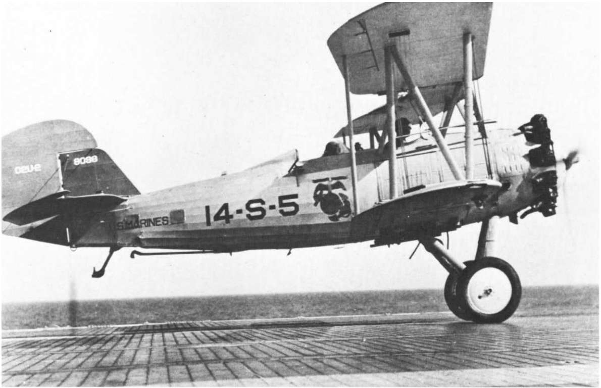
Marine aviation joins the carriers. A Vought O2U-2 of VS-14M on the deck of the USS Saratoga in November 1931. The arresting hook can be seen underneath the fuselage. (Marine Corps Photo 529593).
