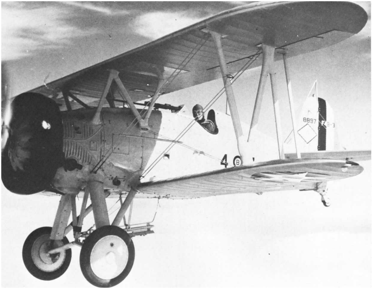
F4B-3 of Bombing Squadron 4 (VB-4M) in flight in 1935. Equipped for dive-bombing, this aircraft had a bomb rack under the fuselage. (Marine Corps Photo 529974).
