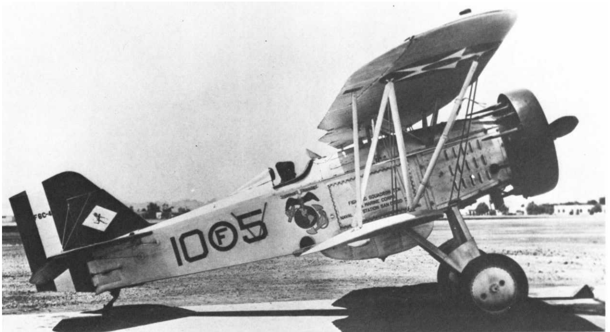
This F6C-4 of Fighting Squadron 10, about 1930, at San Diego has a cowling fitted over the exposed cylinders of its radial engine. (Marine Corps Photo 530812).
