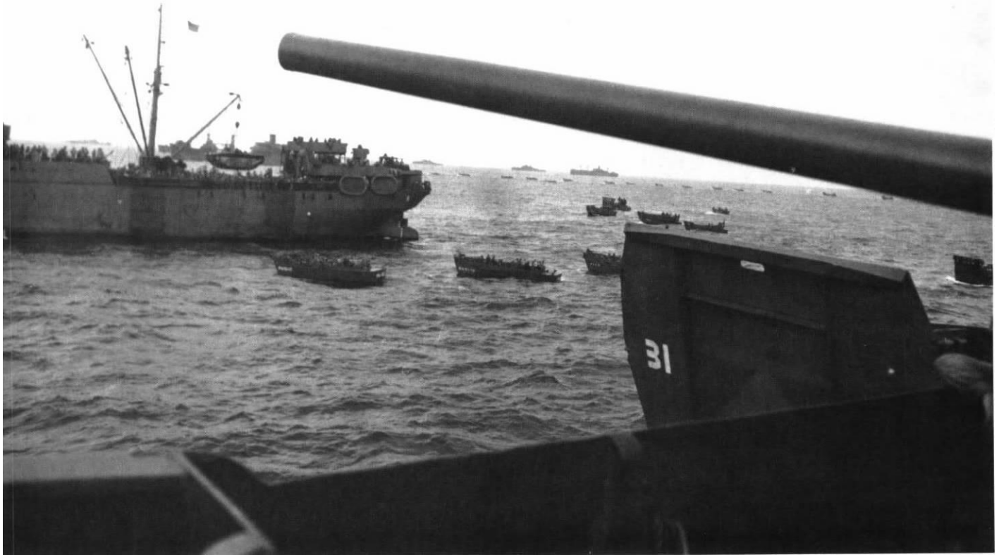
Heywood (APA 6) lowers an LVT-1 by swinging boom in process of debarking assault troops of the 2d Battalion, 8th
