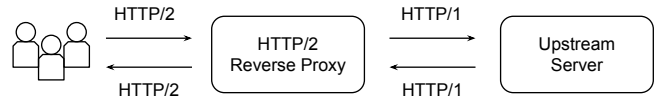
Figure 1: HTTP/2 is used only between end users and HTTP/2 servers. Usually, HTTP/1 is used when sending requests to the upstream servers.
