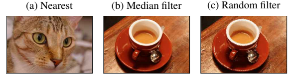
Figure 11: Examples of our defense: (a) insecure nearest-neighbor scaling, (b) robust scaling using a median filter, and (c) a random filter. Note that attack traces are not visible anymore.
