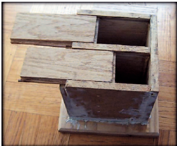
Fig 8. Top of the tank, hatches and partition.
