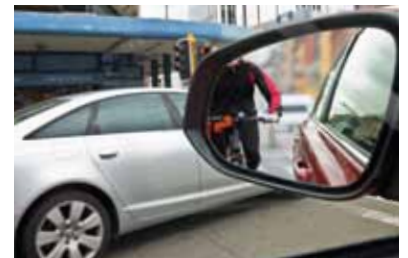
RAV4 Limited is fitted with a Blind Spot Monitor (BSM) that uses radar sensors to detect other road users that may be in your blind spot, a warning light appears in the mirror closest to the object.
