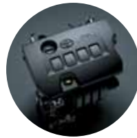
Petrol 2.0 Litre 4 cylinder DOHC with Dual VVT-i and Electronic Fuel Injection (EFI)
