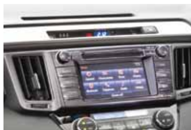
A centre air vent mounted on top of the instrument panel directs air towards the rear occupants to ensure a comfortable climate throughout the cabin.
