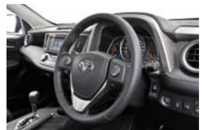
All RAV4 models are conveniently equipped with steering wheel mounted audio controls and have Bluetooth hands-free phone capability together with audio streaming and voice recognition. In the lower instrument panel all models add an additional auxiliary jack and USB input for portable music player connectivity.
