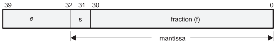
Figure 3–1. Extended-Precision Register Floating-Point Format
