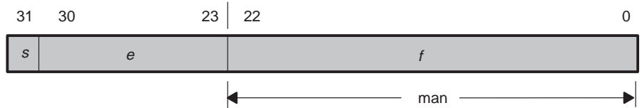
Figure 5–13. IEEE Single-Precision Std. 754 Floating-Point Format
