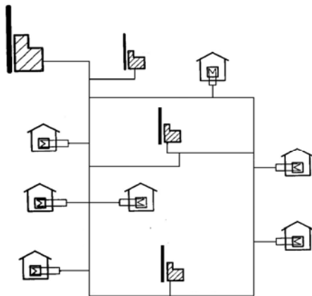
Picture 15. Principle of district heating system in Finland /4, p. 17/.
