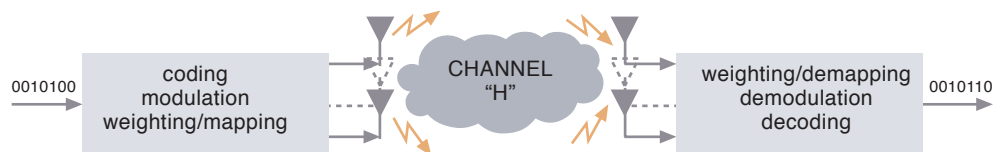
Figure 1 Diagram for a MIMO wireless transmission system. The transmitter and receiver are equipped with multiple antenna elements. Coding, modulation and mapping of the signals onto the antennas may be realized jointly or separately
