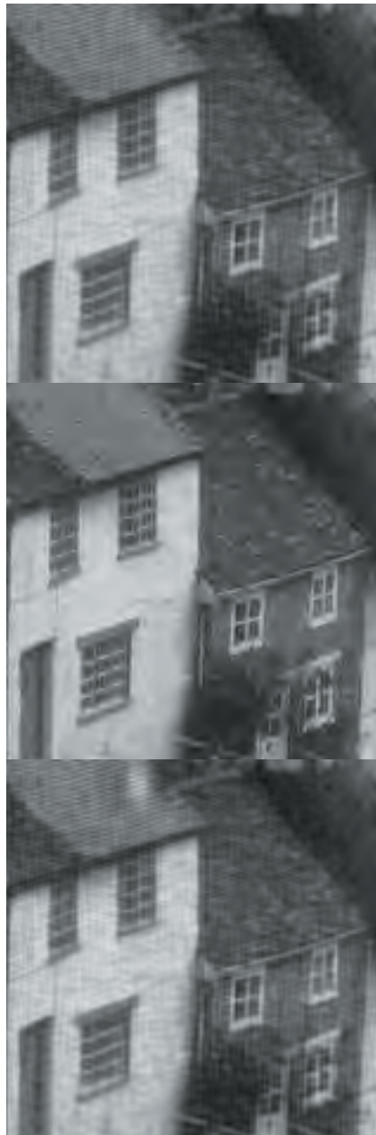
Figure 19 Image coding examples at the rate 0.1 channel symbols per pixel. Upper and lower images result from the proposed coder at CSNR = 20 dB and 17 dB, respectively. The middle image is by the reference coder at CSNR = 20 dB
