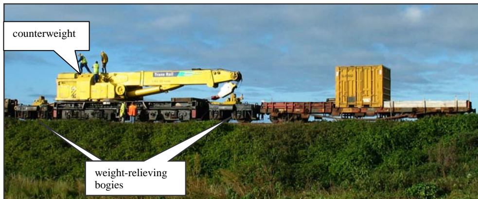
Figure 13 A 60 t rail crane and attendant wagon
