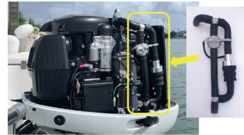
Outboard motor installed with Micro-Plastic Collecting Device
