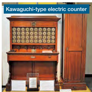
Kawaguchi-type electric counter and turtle-shaped puncher
