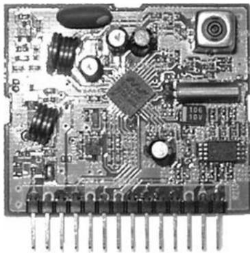
**Fig. 3** FM/AM tuner board using analog-centric CMOS IC.
