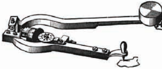
Figure 1.6 The planimeter: a mechanical integrator.
