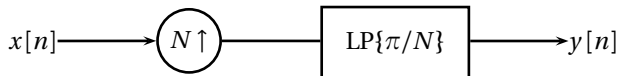
Figure 11.12 Interpolation after upsampling. The interpolation filter is equivalent to a lowpass filter with cut-off frequency \pi/N .
