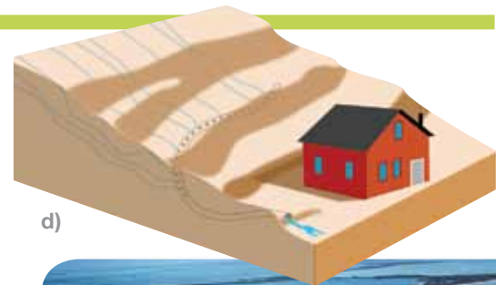
Figure 1–4. (a) Houses and roads are damaged when soils shrink and swell. (b) Buildings in permafrost can shift when the soils thaw and refreeze. (c) Road construction sometimes involves bringing in sand and removing poor local soil. (d) Interceptor drains are used to divert water from foundations. (e) Construction on organic soils requires special engineering to ensure stability. (f) Septic systems in mounds are used to avoid high water tables.
