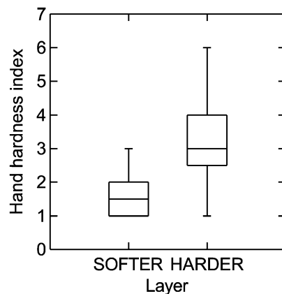
Fig. 17. Hardness in layers adjacent to failure interface. Hardness difference is shown by pair-wise sorting the data ( N = 45 ).
