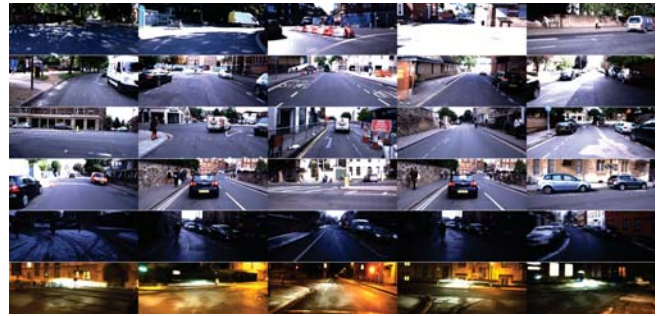
Fig. 6: Incremental changes of lighting conditions in the Oxford10k dataset from early morning (top row) to late night (bottom row).
