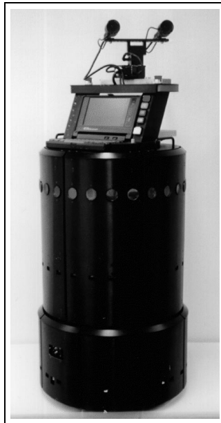
Figure 1. The robot RHINO, an RWI B21.
