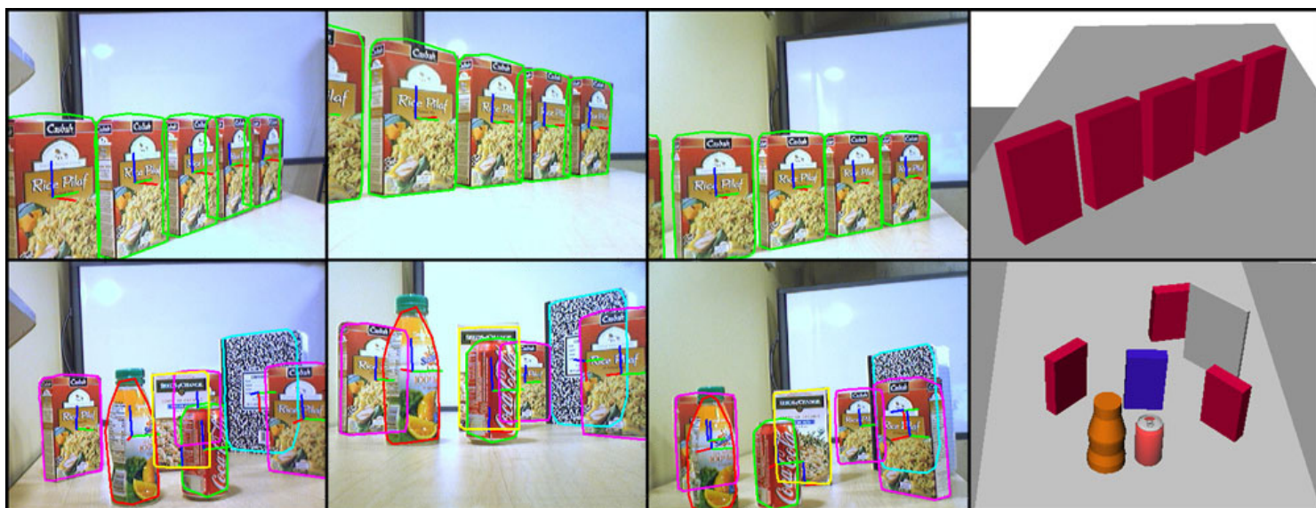
Figure 17: Performance of MOPED-3V in complex scenes. (Cols 1-3) depict the recognized poses overlaid on each image. (Col 4) shows a reconstruction of the given scenes in our virtual environment.
