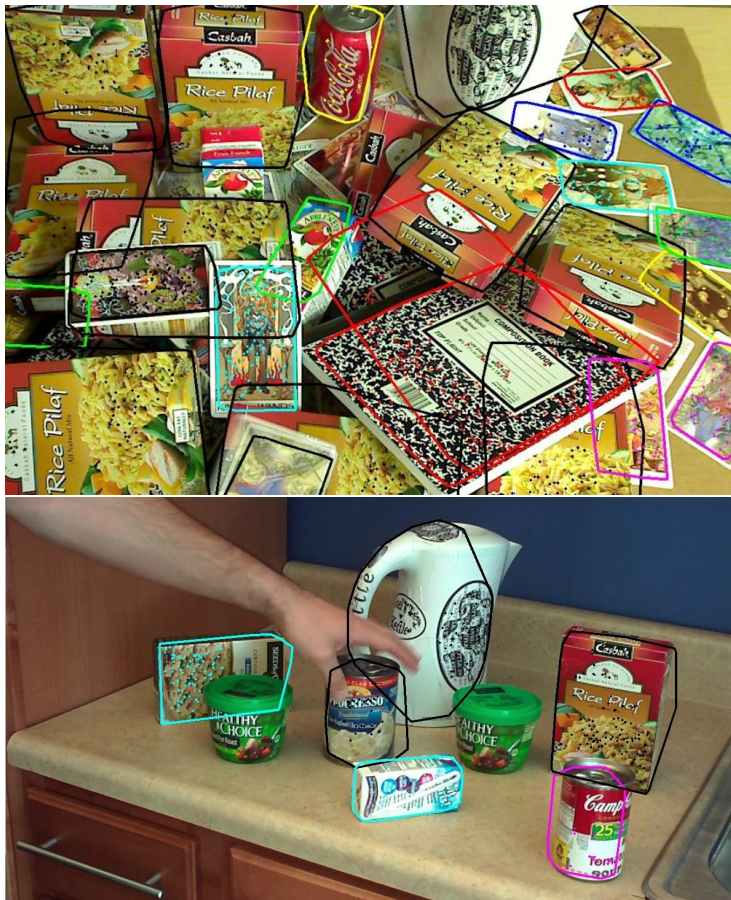
Figure 1: Recognition of real-world scenes. (Top) High-complexity scene. MOPED finds 27 objects, including partially-occluded, repeated and non-planar objects. Using a database of 91 models and an image resolution of 1600 \times 1200 , MOPED processes this image in 2.1 seconds. (Bottom) Medium complexity scene. MOPED processes this 640 \times 360 image in 87 ms and finds all known objects (The undetected green soup can is not in the database).
