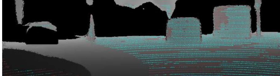
(b) The voxels evaluated as part of the static map, when using semantic-aware evaluation. The ground truth measurements corresponding to the dynamic object not yet being reconstructed are no longer taken into account.
