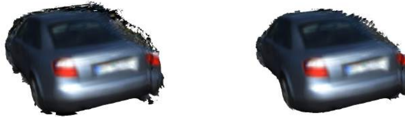
Figure 5.19: Reconstructed car before and after voxel garbage collection (DispNet depth maps). Note the clearer reconstruction border in the right image.
