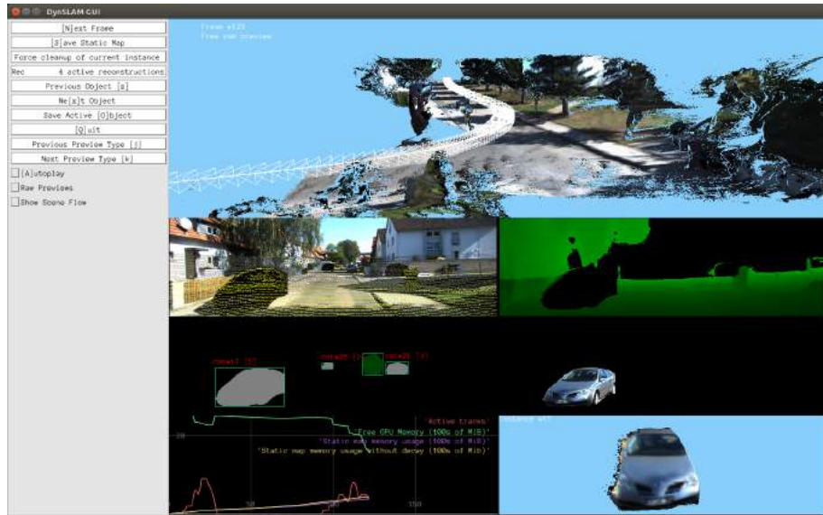
Figure 5.3: The DynSLAM GUI application allows the map and the dynamic objects to be visualized as they are reconstructed. Here, we see a preview of the KITTI-odometry sequence number 5 being reconstructed, around frame 2050. From top-left to bottom-right, it shows (1) a full preview of the active reconstruction together with the camera pose history, (2) a preview of the left camera’s input with the LIDAR ground truth superimposed as a sanity check, (3) the reconstructed depth map with all car silhouettes removed, (4) a preview of the frame segmentation result, (5) a preview of the instance-specific color frame for one of the active reconstructions, (6) memory usage statistics, and (7) a novel view of one of the objects being reconstructed separately from the static map.
