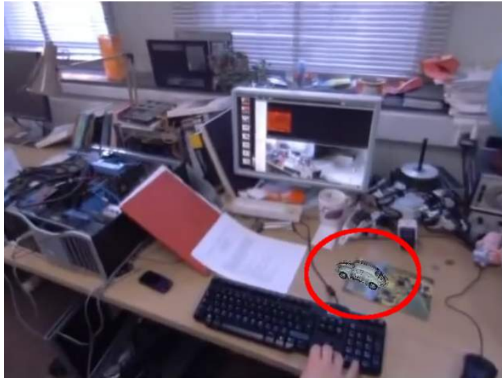
Figure 3.4: An augmented reality vehicle simulation using a dense map created by the Dense Tracking and Mapping system [54] to achieve realistic physics. This highlights one of the many possible applications of dense SLAM systems.
