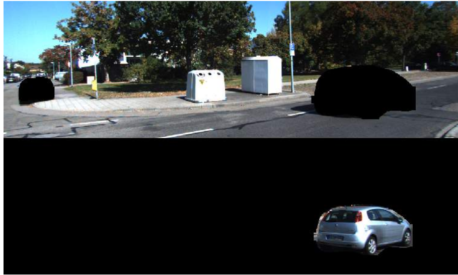
Figure 4.3: The static component of the background is separated from the object instance color and depth frames. On top, we see a sample color frame where a potentially-dynamic and a dynamic vehicle were extracted from the static background while below, we see the corresponding extracted frame for the dynamic vehicle.
