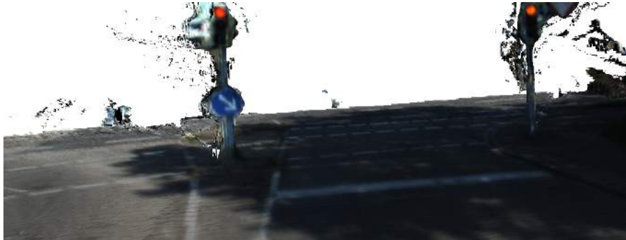
(b) Dynamic fusion, the primary operating mode of DynSLAM, prevents vehicle trails and leftover halos from being integrated into the map.
