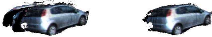
Figure 5.18: Reconstructed car before and after voxel garbage collection (DispNet depth maps). This particularly challenging case was subject to strong motion, and erroneous measurement fusion for the first two frames of the track, leading to the heavy noise to the left of the car. The garbage collection is able to remove nearly all associated artifacts.
