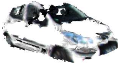
(a) ELAS depth maps are generally accurate, but unable to deal with reflective or transparent surfaces well, leading to less complete vehicle reconstructions.
