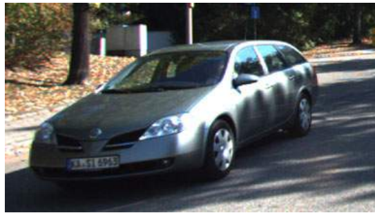
Figure 5.22: Sample car which the direct alignment method fails to track. Note the pronounced reflections on the windows and hood, as well as the shadow patterns on its side. Moreover, despite being quite close to the camera, the featured vehicle occupies an area of roughly 350 \times 200 pixels, less than 10% of the entire frame.
