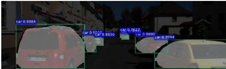
(c) Instance-aware semantic segmentation computed by the MNC [13] architecture. Note that while the segmentation is not dense, and e.g., background pixels are not labeled, the different object instances are well-separated and labeled semantically.
