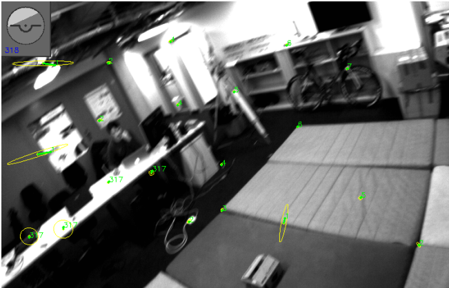
Fig. 2. Screenshot of the running visual-inertial odometry framework. The 2\text{-}\sigma uncertainty ellipses of the predicted feature locations are in yellow, whereby only features which are newly initialized (stretched ellipses) and features which re-enter the frame have a significant uncertainty. Green points are the locations after the update step. Green numbers are the tracking counts (1 for newly initialized features). In the top left a virtual horizon is depicted.
