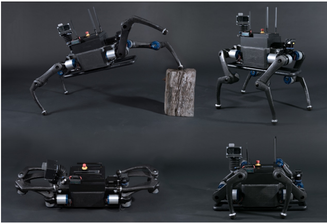
Fig. 4. Full rotation in all joints of ANYmal allow for various configurations.
