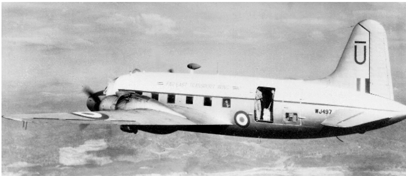
A Valetta displaying the door used for the despatch of paratroops or supplies; this one, WJ497, belonged to the Far East Communications Sqn and was operating over Malaya. (Peter H T Green)
