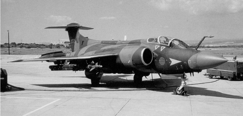
One of the Op PULSATOR Buccaneers at readiness with an LGB and an ALQ-101 ECM pod visible under the starboard wing. (G R Pitchfork)
