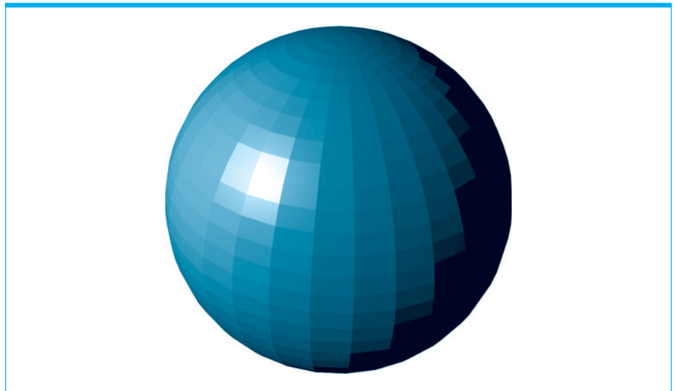
Figure 10.12 A sphere as it might appear when rendered by flat shading
