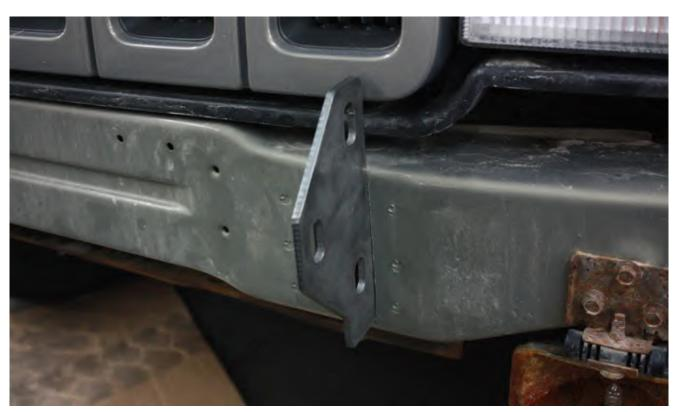
17. At this time you can bolt the Bulkhead Mounts (8) into place and drill the holes need to mount them to the front bulkhead assembly.
