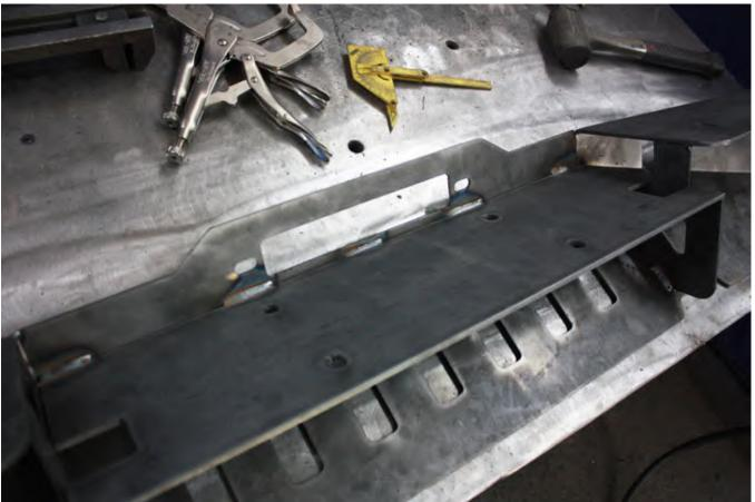
9. Now that the entire bumper is tacked together, it's time to fully weld and grind the bumper!
