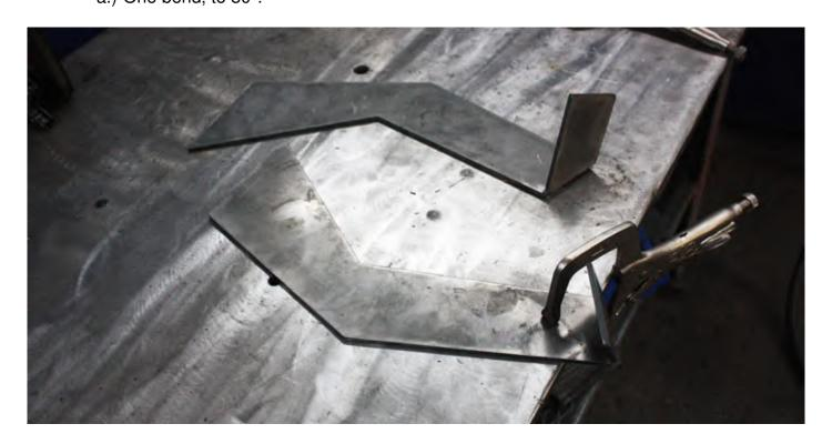
5. With all of the Bumper Parts Bent, it's time to start tacking things together!
