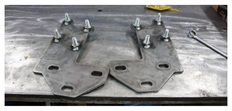
14. Set the Frame Mounts off to the side and grab the Bulkhead Mounts (8).
