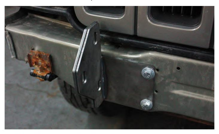
18. On the ends of each side of the factory bulkhead are two pinch seams. These seams will need to be bent over before fitting the bumper. As shown with the red lines below, bend the lower seam underneath and the front seam over to the front.
