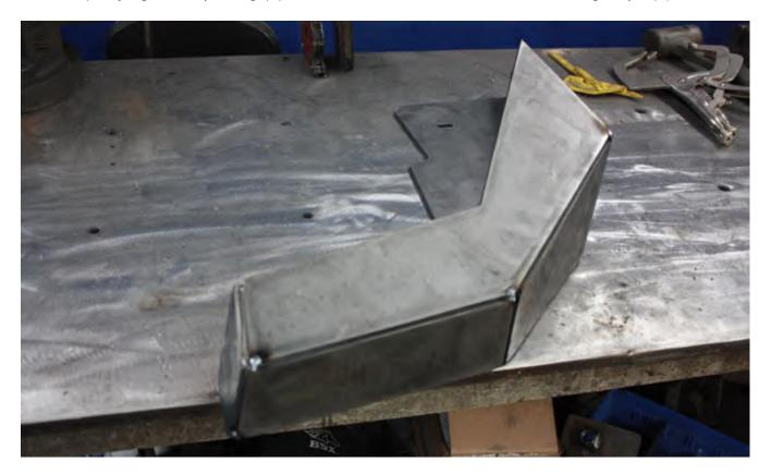
6. Next, lay the Center Section (1) face down on the table. Position the left and right wings as pictured below and tack weld them to the Center Section (1).
