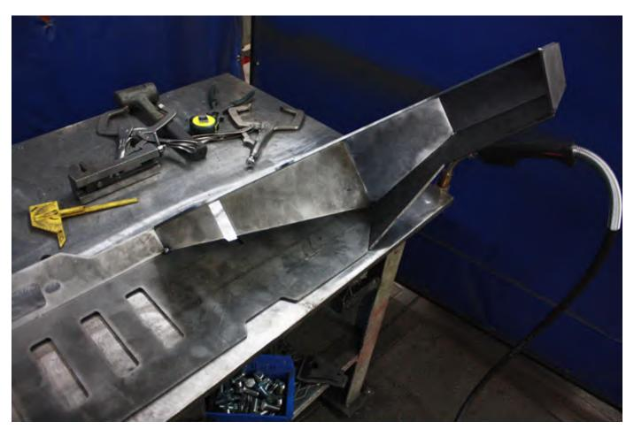
7. Shown below is the Center Section (1) with both left and right wings tack welded in place.
