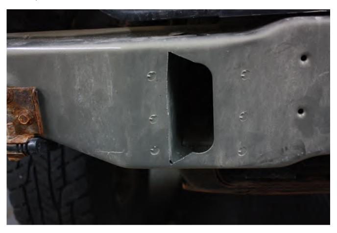
16. Tests fit the mounts and trim more where necessary.
