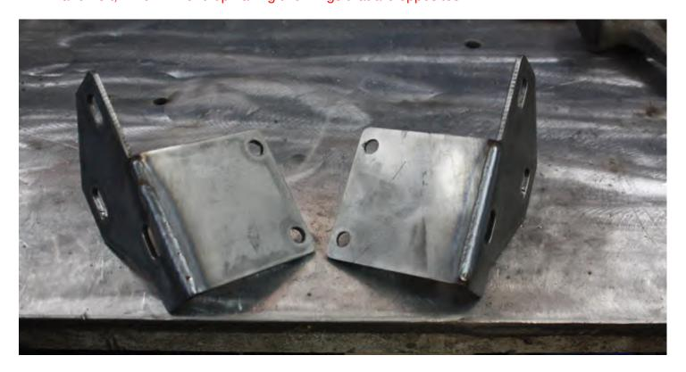
15. In order to install the Frame Mounts (7), you will need to open up the front oval holes in the factory bulkhead.
