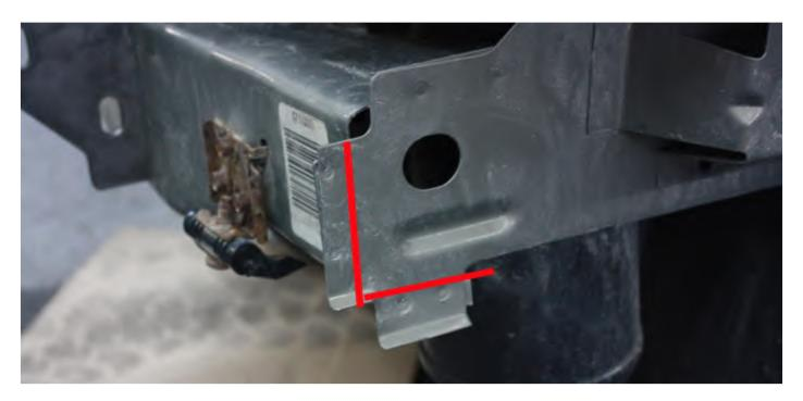
19. With the Frame Mounts installed and bulkhead seams modified, you may now test fit the bumper! Once you have verified the mounting brackets lining up correctly with the frame mounts, you can finish welding the Dring Tabs and Bumper mounts into place!
