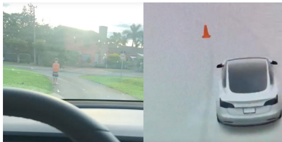
Tesla’s “fix” for the orange barrel problem caused a new problem: the recognition of children wearing orange shirts as traffic cones.
