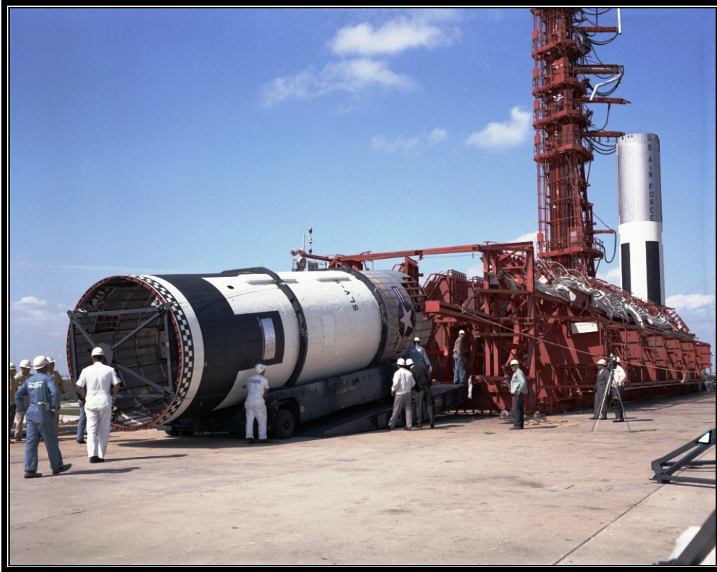
Figure 42. First and second Titan stages being erected at LC-20 (USAF 1964b).
