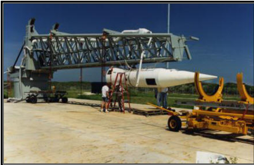
Figure 14. Prospector-1 being assembled on launcher at LC-20 (Bionetics 1990a).
