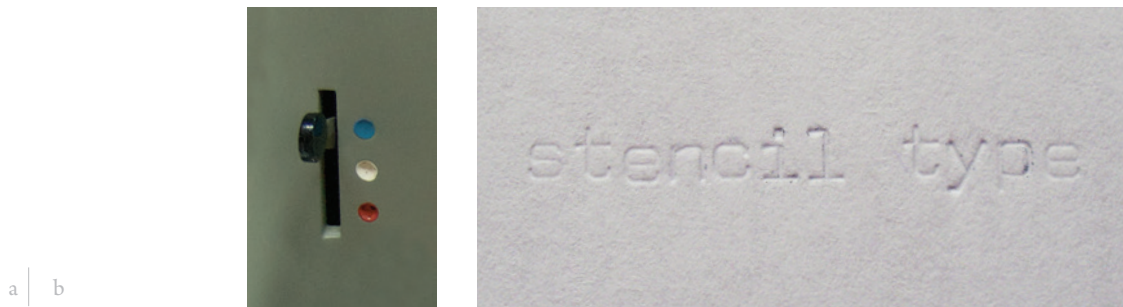
Fig. 54 - a. Colour selector in a Lexicon 80, the white circle is the option for stencil type. b. Close-up of a text sample typewritten in the stencil mode.
