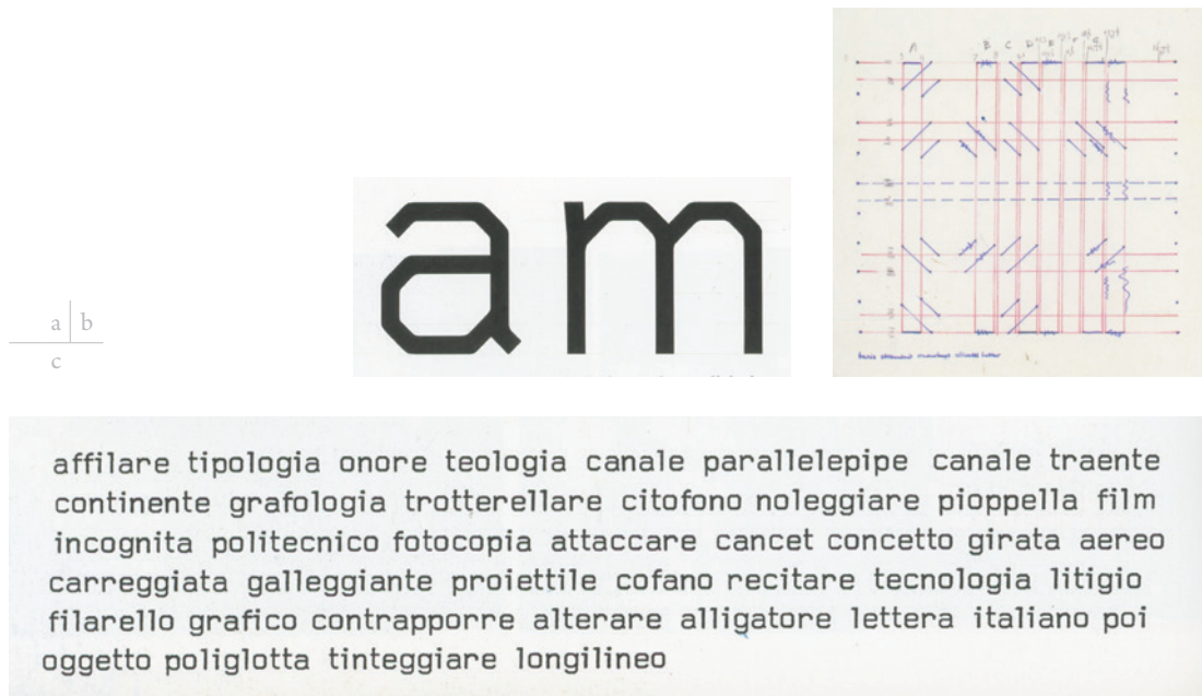
Fig. 22 - Samples of the typeface that Wim Crowel designed for Olivetti. a. Drawings of 'a' and 'm'. b. Grid for the design of the characters. c. Printed proof of the typeface.
