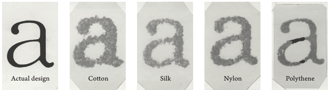
Fig. 27 - Typewritten 'a' printed with ribbons made of different materials.
