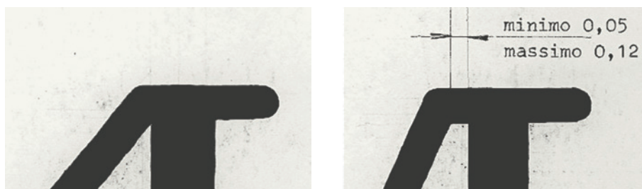
Fig. 30 - Example of how to draw the joints of the strokes in letter 'M'.
