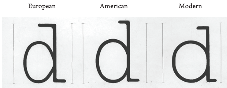
Fig. 58 - Drawings comparing three different designs of 'd' for a Pica typeface.
