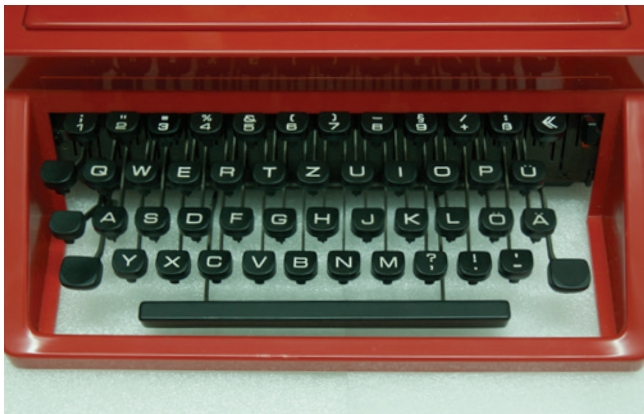
Fig. 10 - The arrangement of the keyboard adapted to different languages and scripts. The character set could also change from one model to another.
