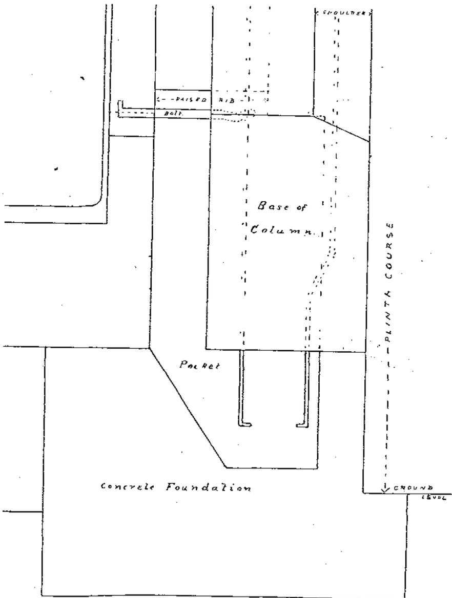
FIG. 3.—Section through Foundations
