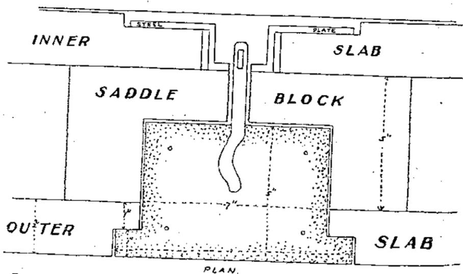
FIG. 2.—Showing Method of Securing Slabs by a Cotter Pin, and Rebating the Outer Slabs to conceal the Columns.
