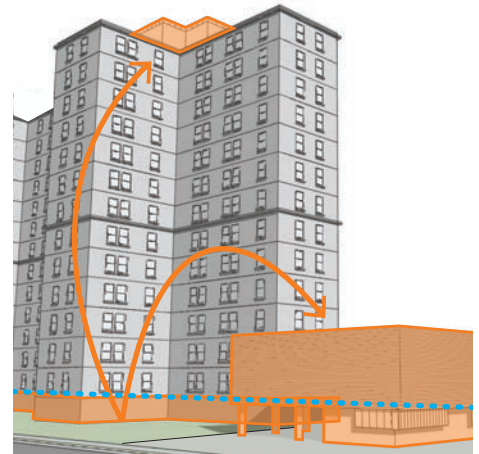
Zoning for Coastal Flood Resiliency Additional flexibility to facilitate mechanical, electrical and plumbing equipment to be placed on the roof or in a separate structure
