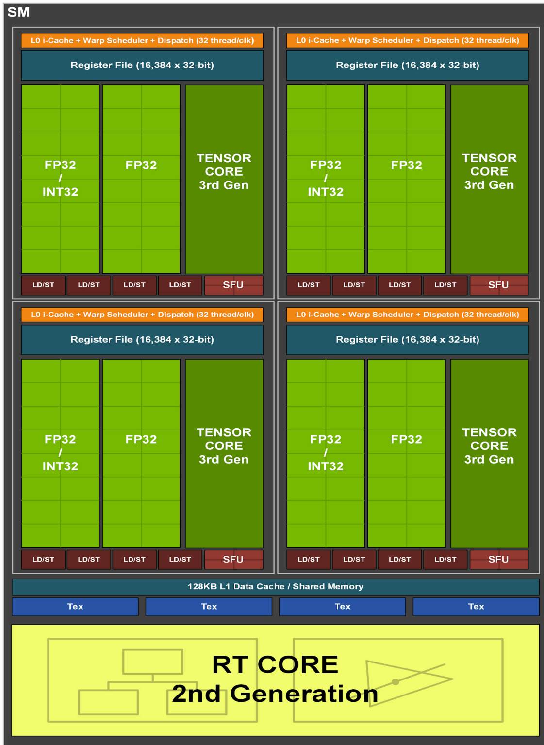
Figure 3. GA10x Streaming Multiprocessor (SM)
