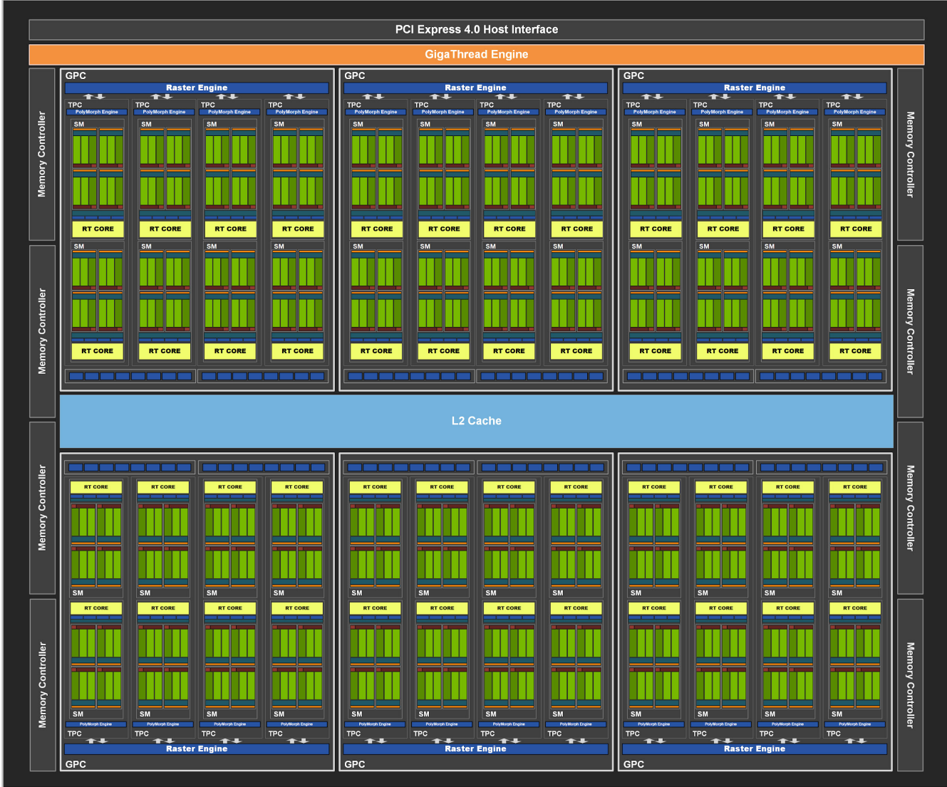
Figure 24. GA104 Full GPU with 48 SMs
