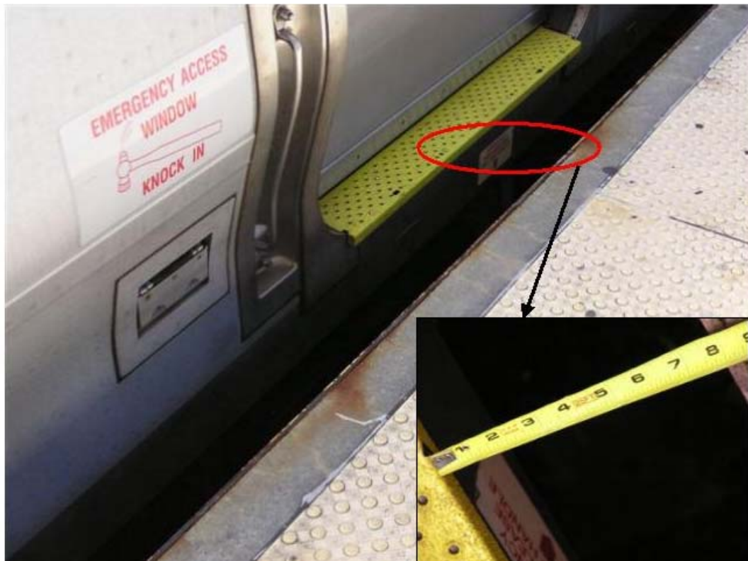
Figure 1. Gap into which passenger fell.
