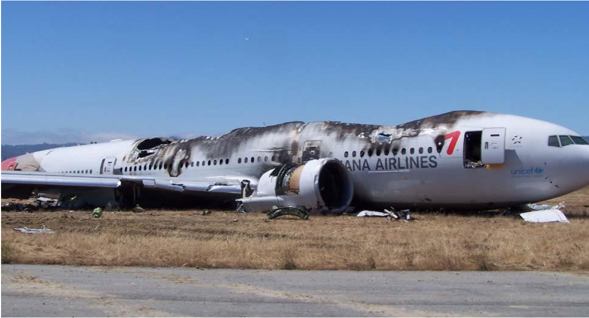
Figure 11. Fire damage to the fuselage of flight 214.
